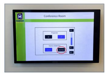
3. After the projector and screen have lowered, push the "Wall Plate" button under the "Source Selection" heading. Plug the other end of the HDMI cord into your laptop.
