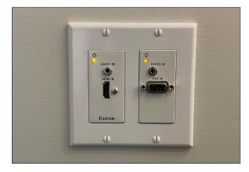
1. Plug an HDMI cord into the HDMI port on the wall. The port is located under the touch panel next to the whiteboard at the front of the room.
