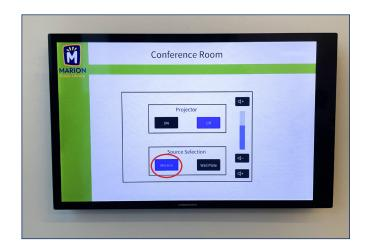
2. After the projector and screen have lowered, push the "Mersive" button under the "Source Selection" heading.
