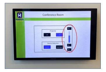
4. The laptop will connect automatiacally to the projector and overhead speaker system. Volume can be controlled with the plus and minus signs on the touch panel.
