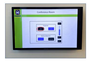
1. Push the "On" button underneath the "Projector" heading to lower the technology.
