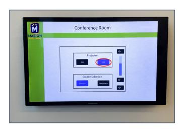
2. Push the "Off" button underneath the "Projector" heading to shut down the projector and screen. This will turn off the technology completely and reset it for the next user.
